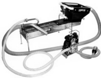
Figure 5. Power sluice/suction dredge combination
